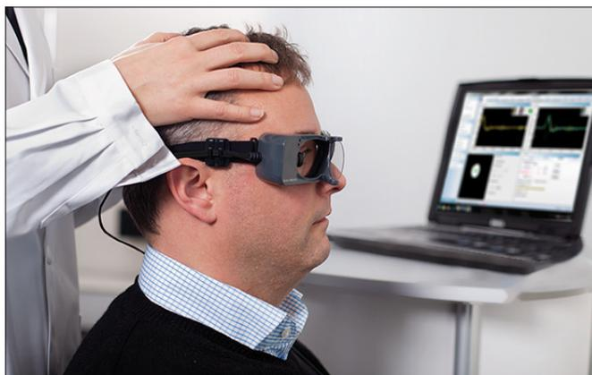
*Caution: Touching the goggles or the goggles strap while moving the patient's head can result in moving the camera which produces artifacts in the collection data.*
