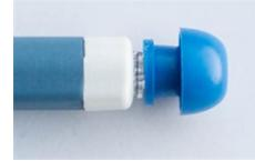
1. Firmly push and twist the eartip onto the probe tip, until it rests firmly against the base of the probe tip.
