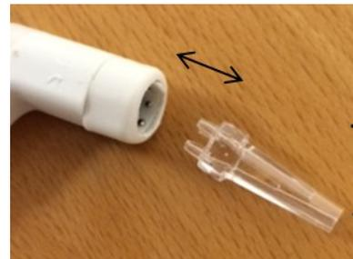
3. Check to see if the sound channels of the probe tip are blocked. You can fit a new probe tip on the probe, or use the supplied probe tip flossing thread to clean the sound channels.
