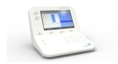
MADSEN Zodiac Quick Check performs automatic 226 Hz tympanometry which can be combined with Ipsi Reflex testing.
